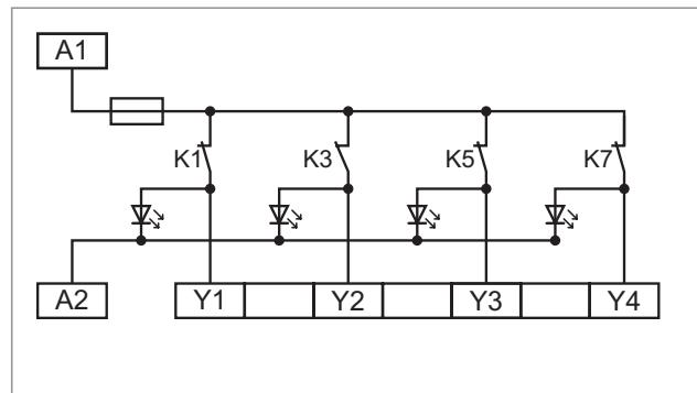
LED's or signalling outputs signalise an opened protective device or emergency stops.
