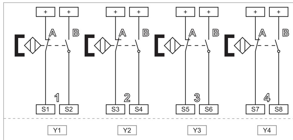
Wire breakage and earth leakage in the control circuits are detected.
