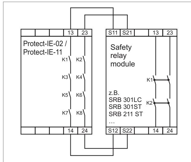
All standard safety relay modules of the SCHMERSAL Group can be connected to the devices Protect-IE-02 and Protect-IE-11.
