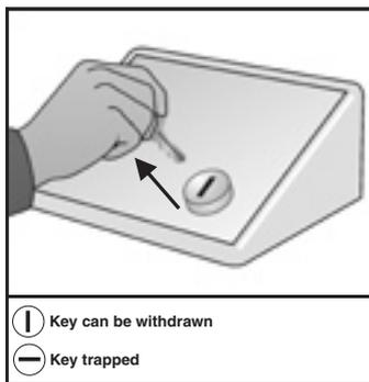
2. This enables the key to be transferred from the key-operated selector switch to the guard.
