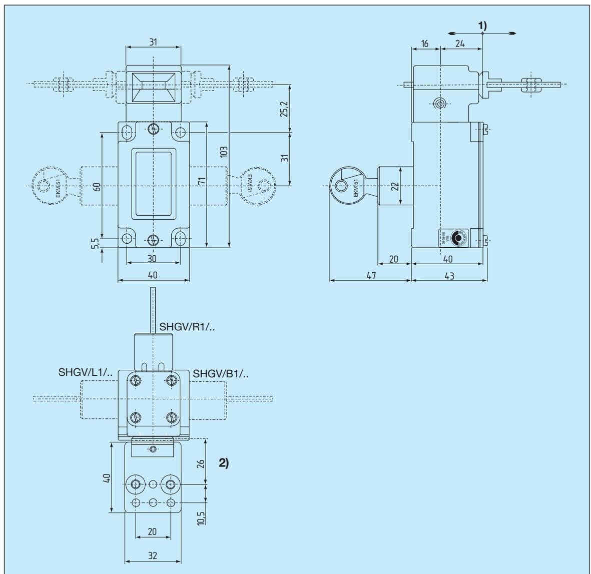
1) Basis of measurement for actuator; 2) Control head set to front by factory
