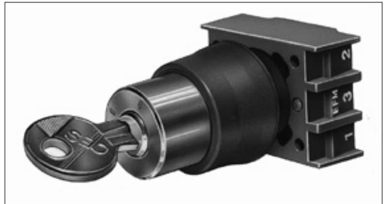
In key withdrawal position S2, the plunger in the operating head positively acts on the contact element and thus positively opens contact 11-12. Two additional contact elements can also be snap fitted to the mounting flange and any contact configurations can be selected.
