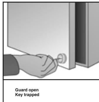
5. A mechanical fail-safe device prevents the key being switched back when the guard is open.
