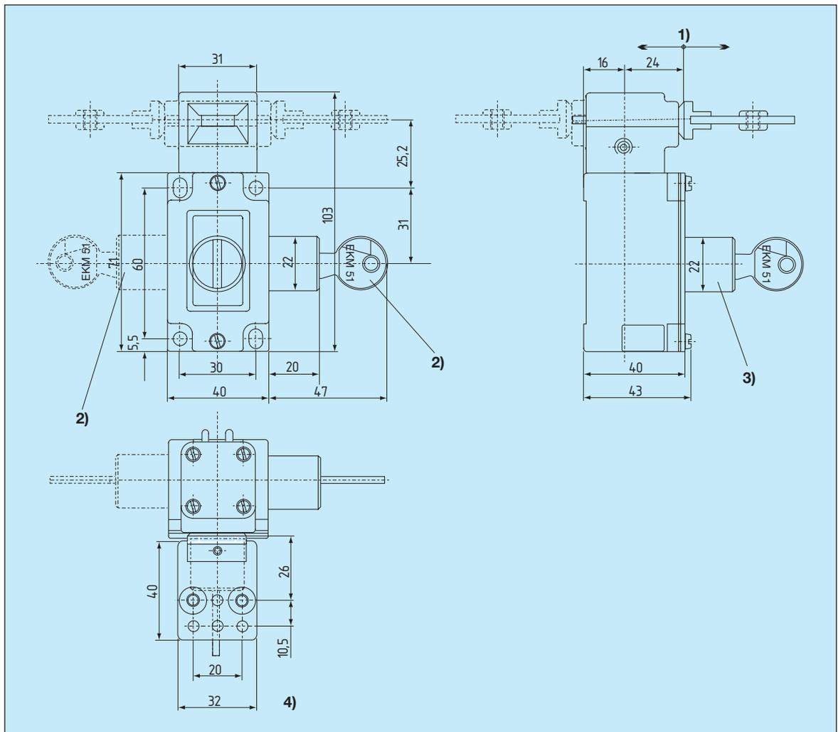
1) Basis of measurement for actuator; 2) Lock barrel 1 (to lock the guard), 3) Lock barrel 2 (to lock barrel 1 when guard open), 4) Control head set to front by factory
